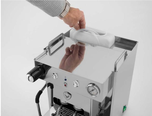
*WE RECOMMEND USING A WATER SOFTENER FILTER OR ANTI-SCALE BAG* that must be periodically replaced. If this is not done, lime deposits may form inside the machine, potentially affecting its proper functioning and voiding the warranty. After inserting the water softener filter into the tank, fill it with drinking water, preferably low in calcium. Use a funnel and a bottle to fill the tank.
