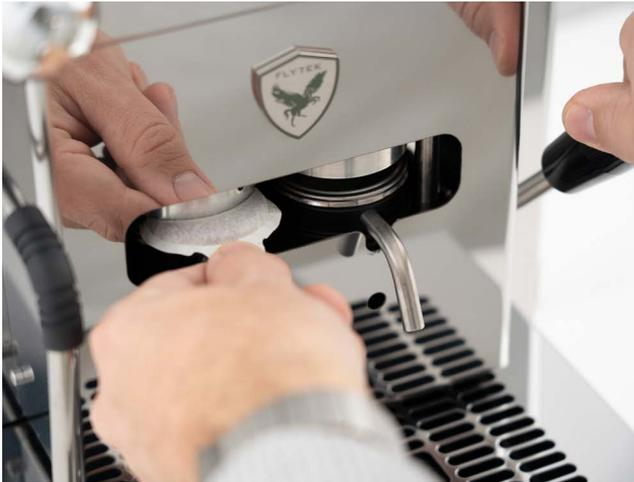
Gently lower the lever until it clicks into place. Place a cup under the spout where the pod has been positioned and press the corresponding coffee pouring switch (ref. D); after approximately 5 seconds, the coffee will start pouring.
